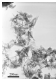
HA (×50,000) Needle ribbon width 240nm minimum width 50nm
